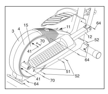
Next, remove the four Screws (51, 70) from the right Pedal Disc (15), and slide the Pedal Disc off. Remove all Screws (52, 64) from the Right Side Shield (4) and the two Bolts (41) from beneath the Pedal Disc, and remove the Right Side Shield (4). Remove all Screws (52) from the Left Side Shield (3), and remove the Left Side Shield.
